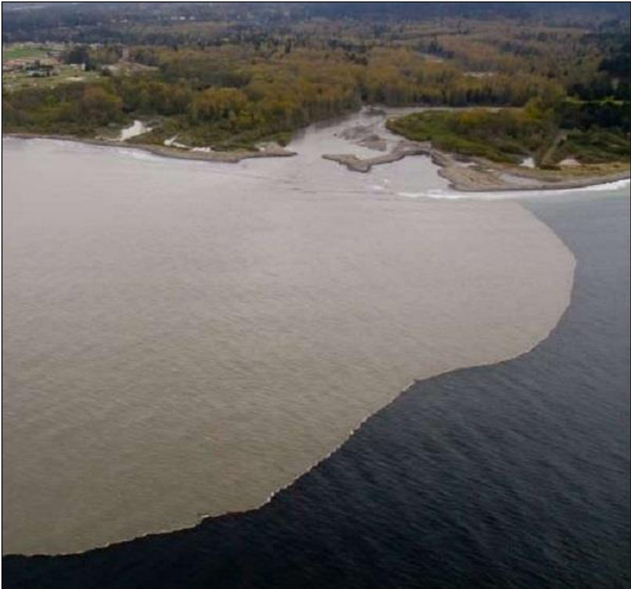
Sediment-laden waters of River Elwha reaching the coastal waters after Elwha Dam Removal. ( http://gallery.usgs.gov/ )
