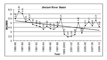
It is clear from the above graphs and analysis that the decline in per MW generation is observed in all the fiver river sub-basins of the Indus Basin. The Indus sub-basin generation is not analysed since in the Indus basin within India, there are only two small hydro projects.
