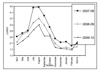
These graphs and figures therein also indicate that the issue of over 89% of operating hydropower projects generating at below the design generation figures and half of them generating below the 50% of design generating capacity remain valid. Moreover, the issue of how much of the power is generated during peaking hours also remain equally valid. These issues were highlighted in earlier SANDRP analysis, for more details, see:
