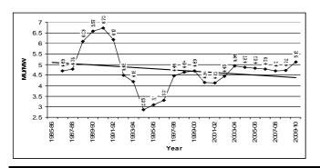
**Jhelum Basin** The operating hydropower projects in Jhelum Basin (736.6 MW) include: Mohara, Gandharbal, Uri, Lower Jhelum and Upper Sindh hydropower projects. The trend-line for generation per MW is again showing downward slope, showing that the generation has been diminishing over the years.
