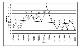
Ravi Basin The operating hydropower projects in the basin (1738.35 MW) include: Chamera I, Chamera II, Baira Siul, Sewa I, Ranjit Sagar and Upper Bari Doab Canal hydro project. The diminishing generation here is more pronounced than in case of Beas basin.
